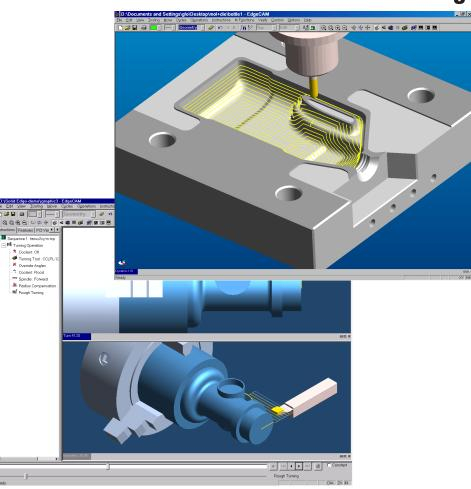
An affordable full industrial CAM package designed by Pathtrace. Offers intelligent manufacturing solutions for production milling, turning, and mold and die making.
