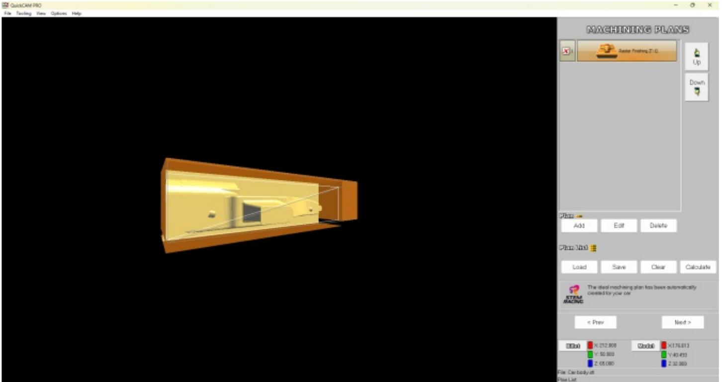
The Car Wizard loads the SRCarPlan.qpp and then automatically generates the cutter path.
