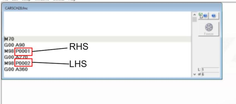
The program with the car name is the Subcall program. This is the one that will be run to cut the car.
