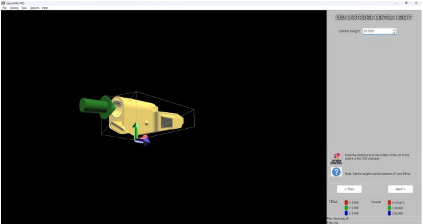
The model will be positioned around a datum position set in the middle of the CO2 Cartridge chamber. The height of this must be recorded when the car is being designed in CAD and to ensure the car can be manufactured in an F1 Model block the value must be between 21mm and 29mm.
