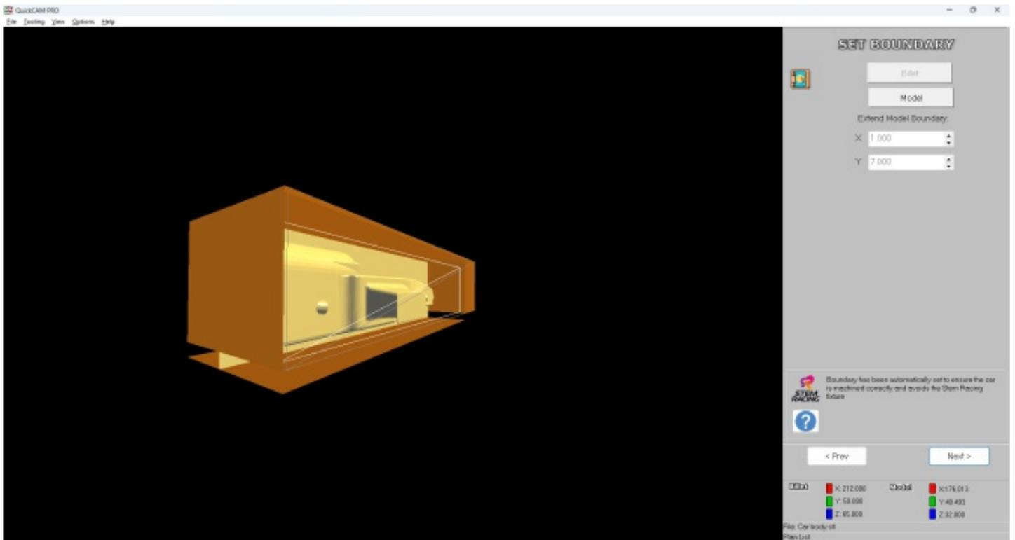
The Boundary is pre-set to allow the tool to travel 7mm outside the block in the Y axis. This is so that the tool has room to be allowed to machine the floor and top of the car.
