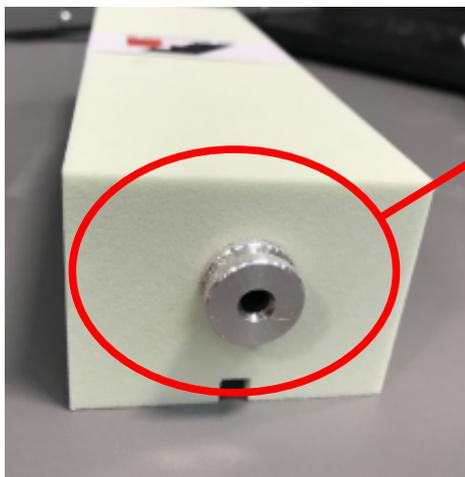
*Aluminium cartridge inserted into the cartridge hole in the billet. Note the hole in the centre, this locates onto the 4th axis tail-stock.*
