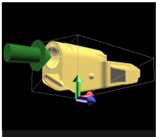
Once the centre height is correctly entered and the green arrow is correctly positioned in relation to the bore the Next button will be enabled. ***This value will be recorded for later use.*** Click the Next button
