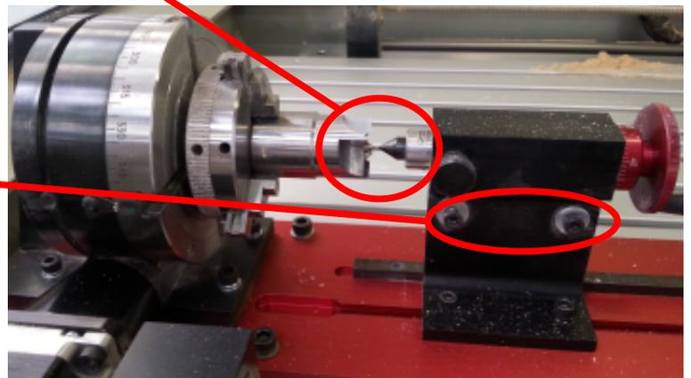
*Use these bolts to loosen the tail-stock in order to align it with the chuck.*
