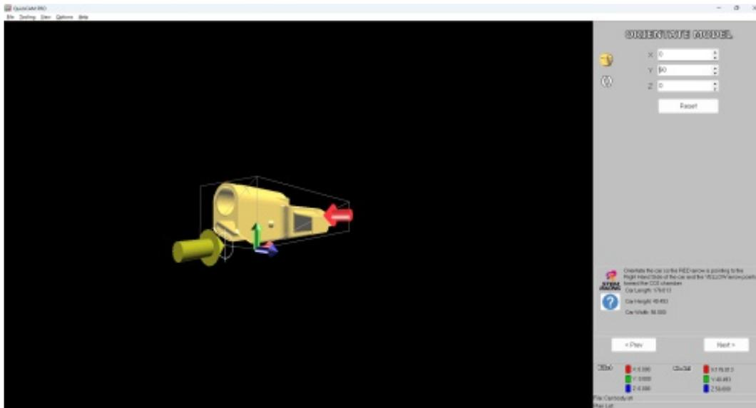
If the model requires rotation click on any of the axes buttons and these will rotate the model in increments of 90 degrees.
