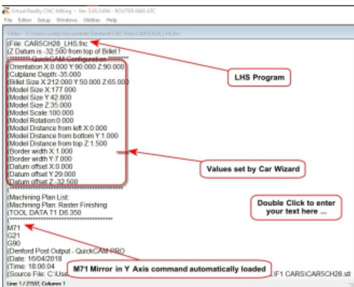
VR Milling Shown with the LHS program Loaded showing the M71 command.
