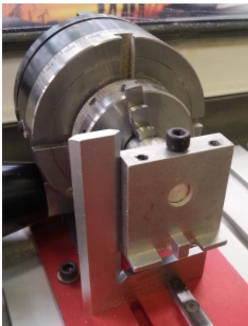
The aluminium block which holds the billet fixes into the chuck of the 4th axis.
