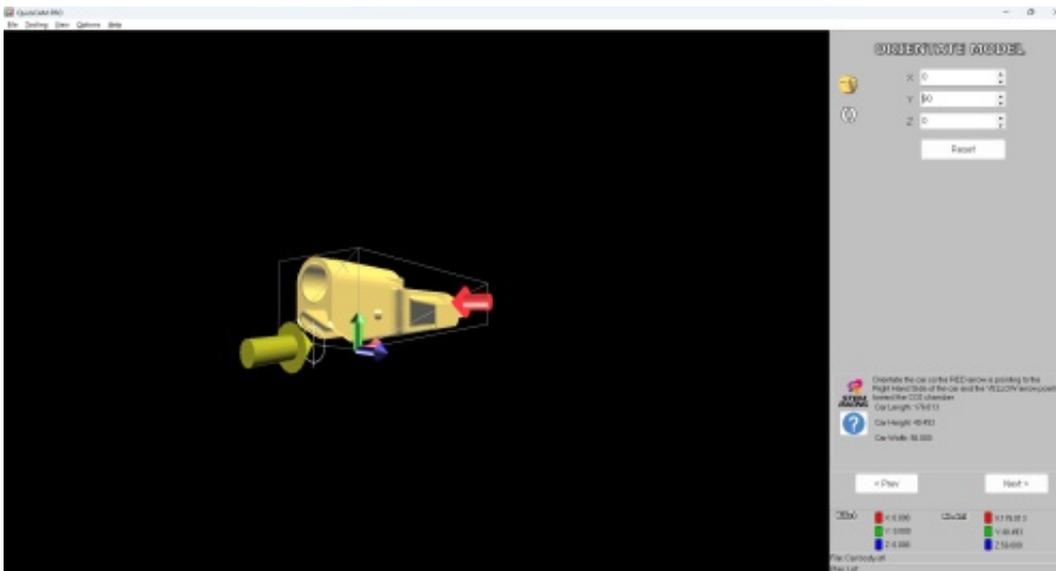
If the model needs to be rotated, click on any of the axes buttons and these will rotate the model in increments of 90 degrees.
