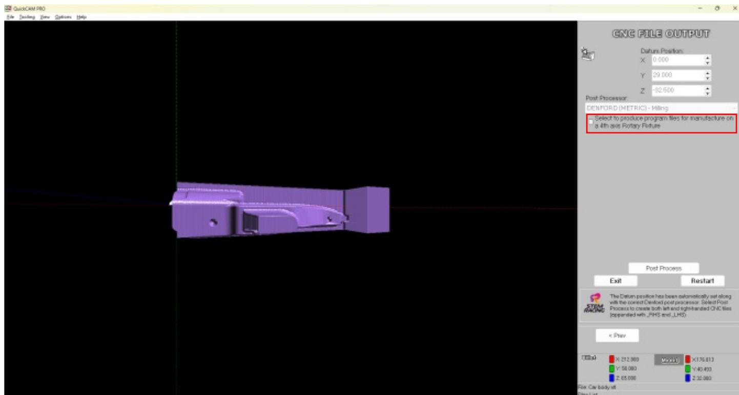
The Car Wizard will automatically set the Datum position at the centre of the CO2 Cartridge chamber
