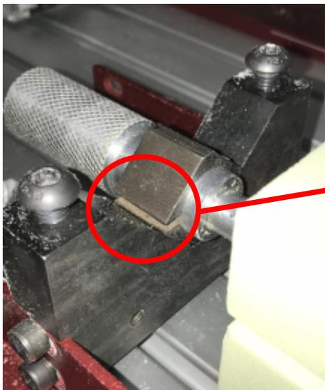
***Always ensure the Billet is pushed as far to the right in the fixture and the front of the car is clamped into position before clamping the shaft at the rear.***
