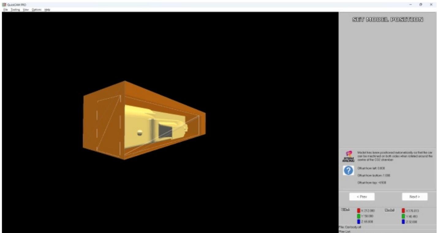
The Car Wizard recorded the width, height and length of the car on the Orientate Model page. The height of the CO2 Cartridge chamber from the base of car was also recorded.
