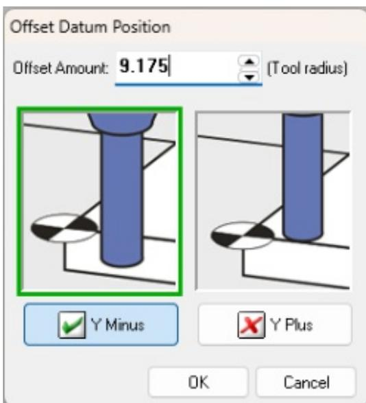
The tool is 6.35mm Diameter so 3.175mm Radius.
