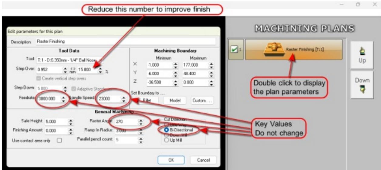
By double clicking on the machining plan the plan Parameters can be displayed.
