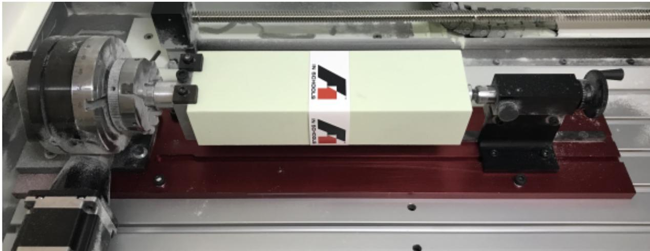
Note that the tether line guide slot is at the bottom closest to the bed of the machine and the cartridge hole is on the right, the cartridge hole should have the aluminium cartridge fitted into it and this mates up to the tail-stock of the 4th axis.
