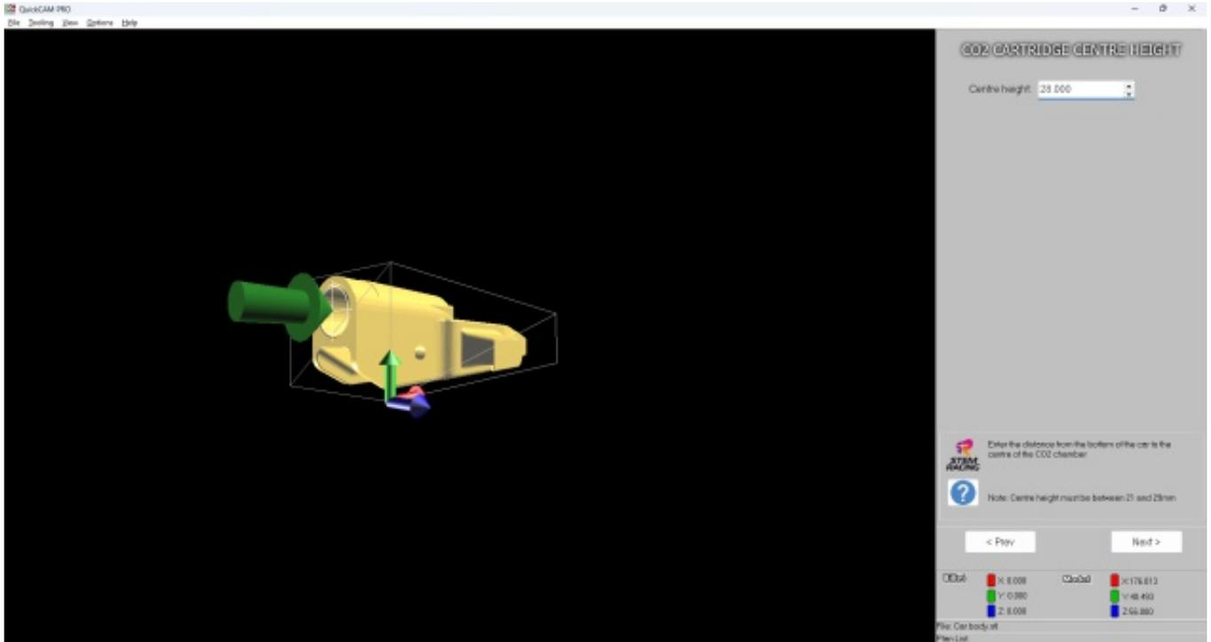
The model will be positioned around a datum position set in the middle of the CO2 Cartridge chamber. The height of this must be recorded when the car is being designed in CAD and to ensure the car can be manufactured in an STEM Racing Model block the value must be between 21mm and 29mm.
