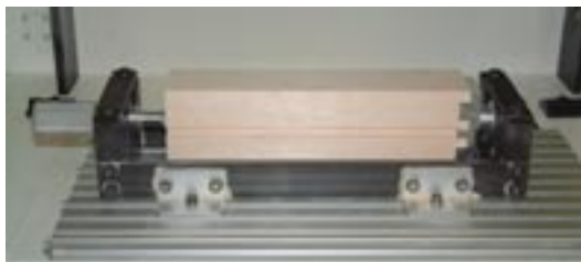
Fit the balsa wood billet in the jig as shown.
