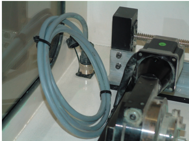
Plug and 4th axis rotary fixture fitted
