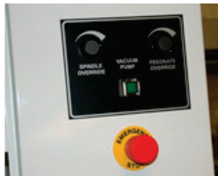
Spindle and Feedrate potentiometers
