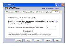
The first screen of the Results tab lists the lowest factor of safety (FOS) of the model under the specified load and restraint.
