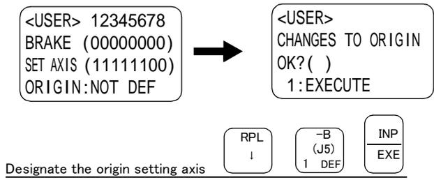
8) Press the [ ↓ ] key, and input “1” for the axis for which the origin is to be set. Press the [INP] key to display the Confirmation screen.
