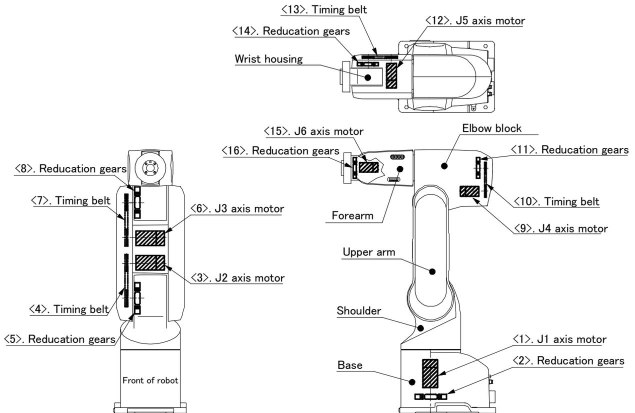
Fig.5-3 : Outline structure drawing of robot arm (6-axis type)
