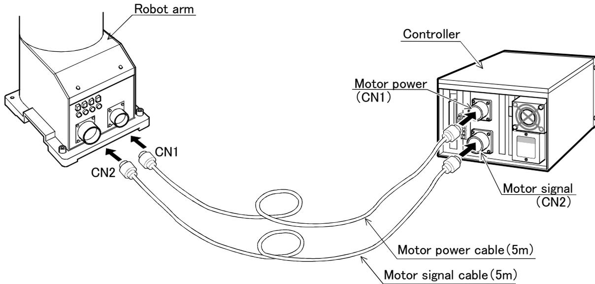
Fig.2-6 : Connecting the machine cables
