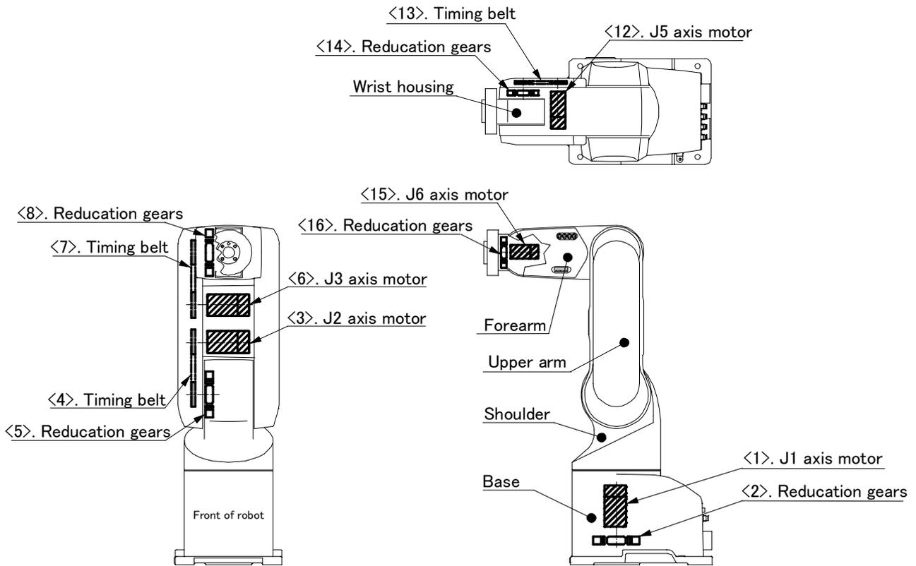
Fig.5-2 : Outline structure drawing of robot arm (5-axis type)
