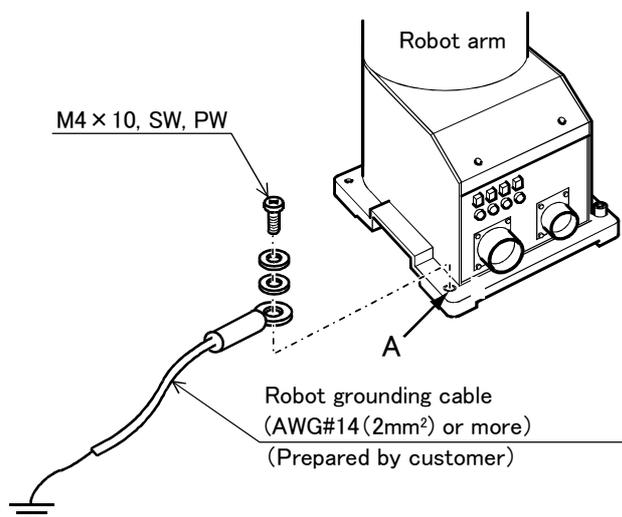
Fig.2-5 : Connecting the grounding cable
