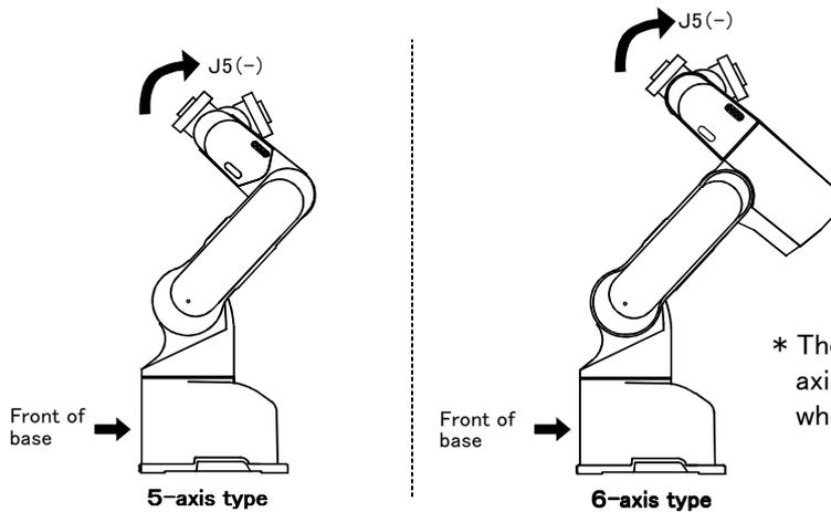
\* The J5 axis direction for the 6-axis type indicates the direction when the J4 axis is at 0° .
