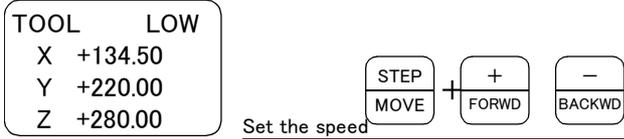
Press the [MOVE] + [TOOL] keys to select the TOOL jog mode. "TOOL" will appear at the upper left of the screen.
