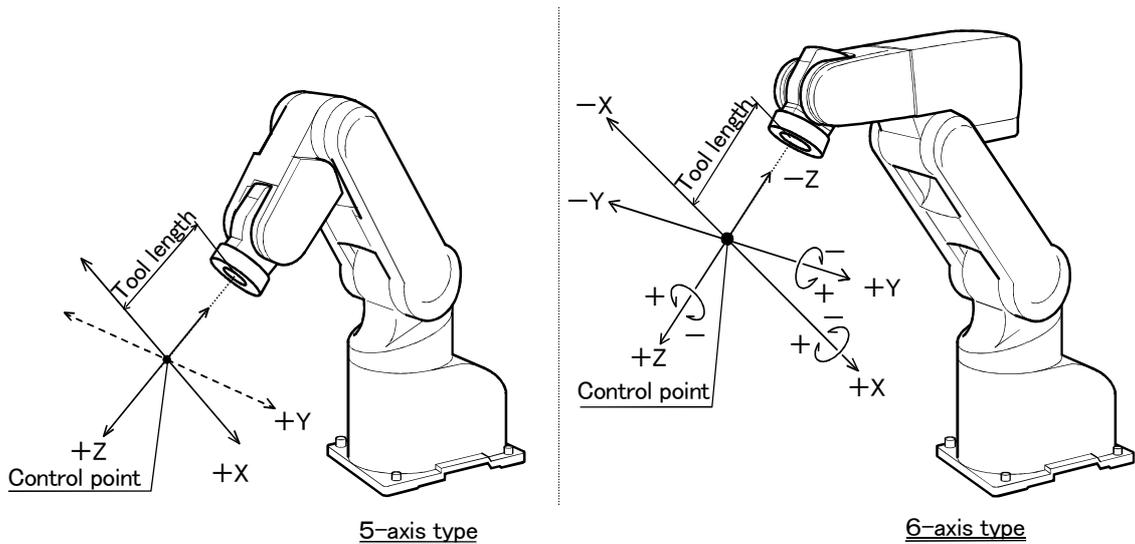
\* While maintaining the flange surface posture, the axis moves straight along the tool coordinate system.
