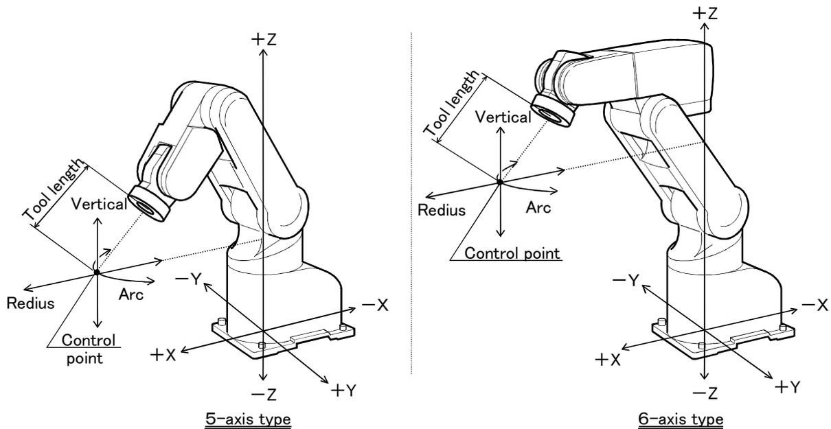
\* The current position is set as the arc centering on the Z axis, and the axis moves along that arc, expands and contracts in the radius direction, and moves vertically. At this time, for the 6-axis type, the flange surface posture is maintained. Also, while maintaining the flange surface position, the flange surface posture changes.
