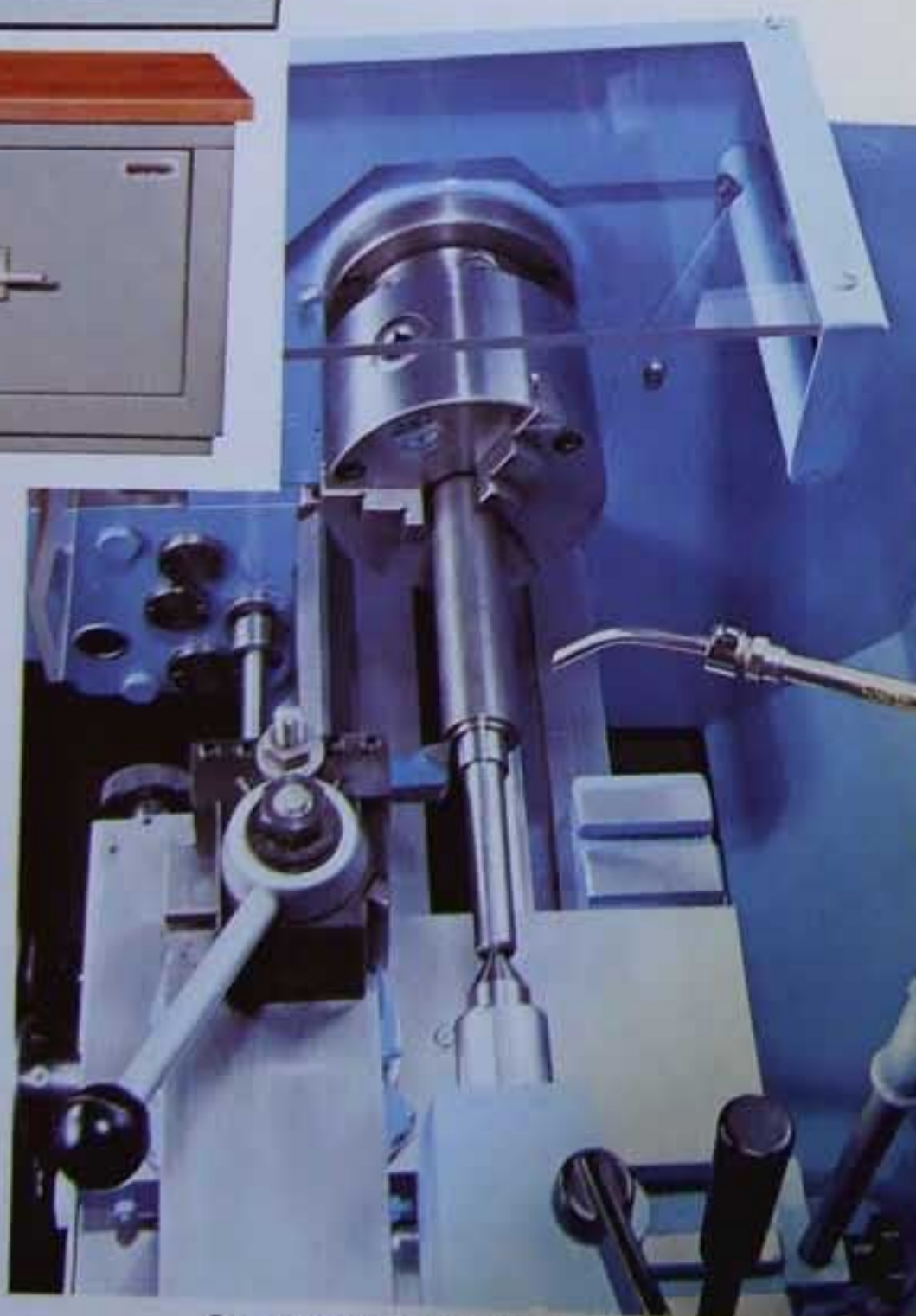
Output, from main camlock spindle showing compact arrangement of saddle assembly.
