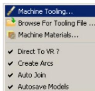
**Machine Tooling** - Opens the Tool and Offset editor
