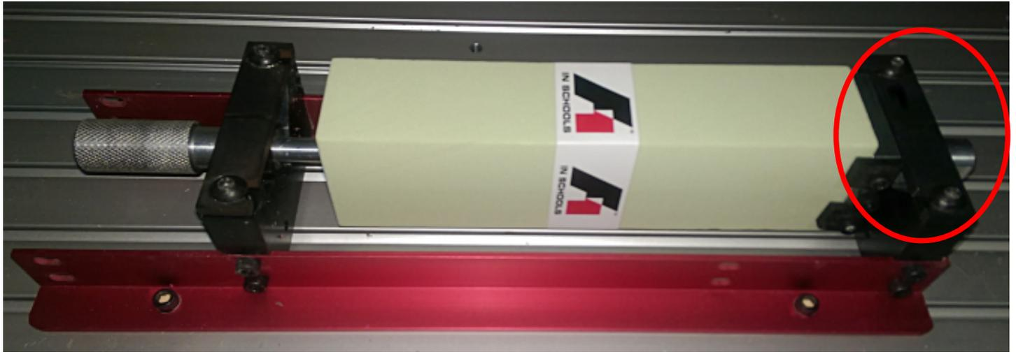
When tightening the bolts circled in the image above always tighten the right hand side before the left to prevent the billet from being twisted.
