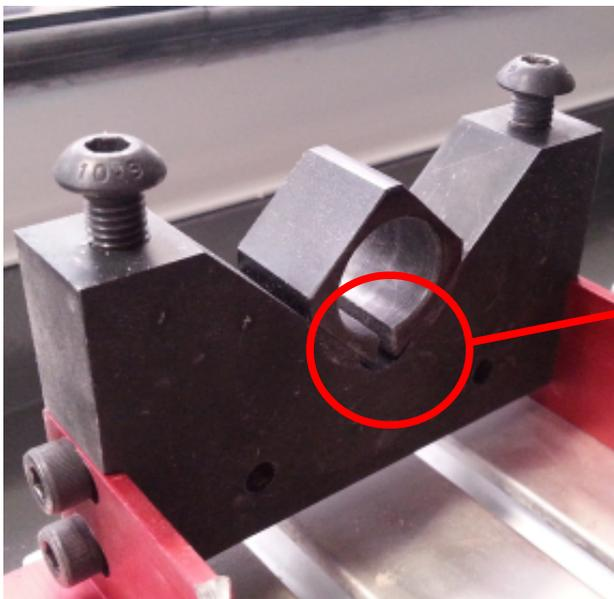
***Ensure that this cutout is at the bottom. As the bolts are tightened onto the aluminium bar that goes over this bracket the cutout closes up and secures the aluminium post which is inserted into the cartridge hole.***
