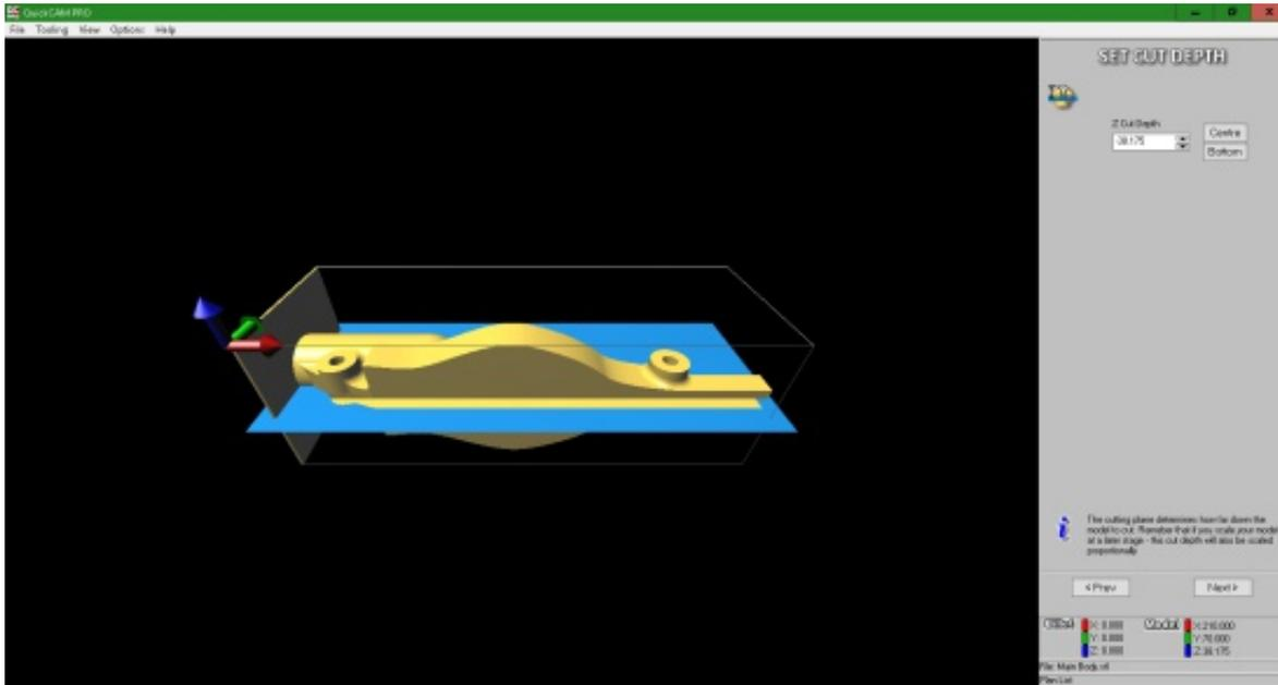
We will be machining the car from the left and the right hand sides, we could set the cut depth to the centre, but as we are using a ball-nose cutter this would leave a ridge down the centre of the model.
