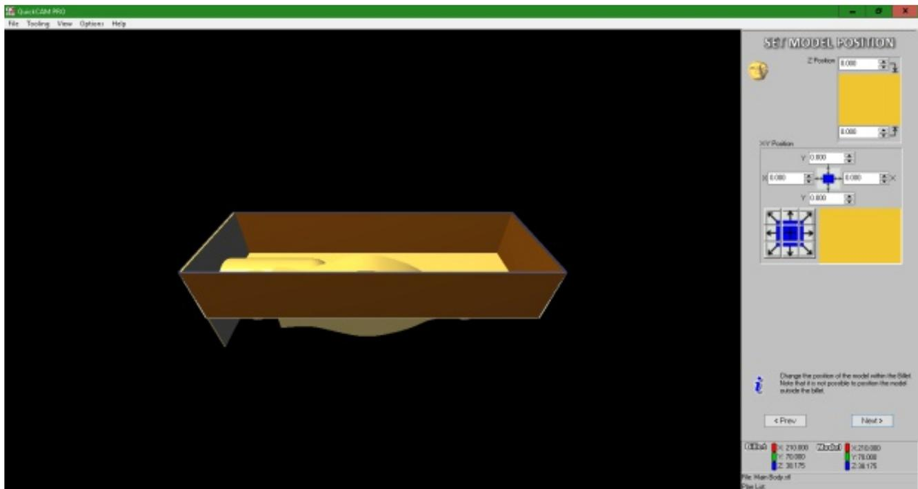
It is very important to get this correct as the cartridge hole is already in the billet and has an aluminium post inserted into it, getting the model position wrong may cause damage to the fixture and possibly break a tool.
