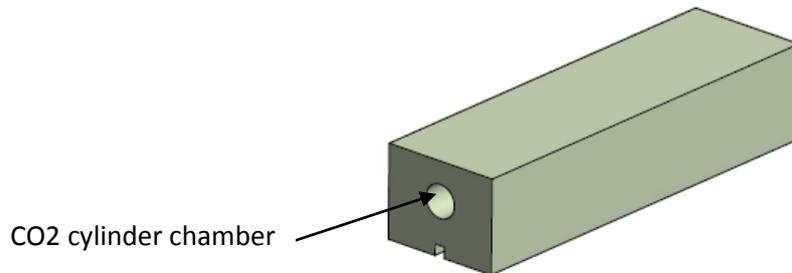
The F1 Fixture and the 4<sup>th</sup> Axis Car Manufacturing Conversion Kit will be changed to fit the F1 Model Block 18mm CO2 chamber bore.
