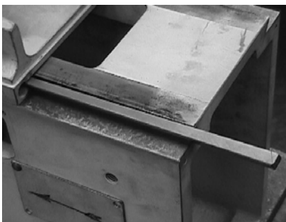
Production of a Novamill machine column, showing the fitting of a Z axis gib strip.
