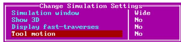
When '*Run Program*' is selected, the tool motion will be shown , throughout the running of the program cycle. The program cycle may run slower with this option switched 'on'.
