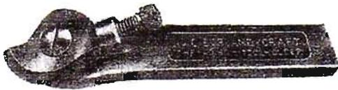
The cam form cutter can be positively adjusted to suit centre height. The cutter is easily re-sharpened by grinding on the top face of the form—the tool-holder is then ready for use again. The cutters are made of High-speed Steel, hardened and ground. Each holder supplied with one Whitworth Form Cutter. Can be supplied with Metric, B.A. or U.S.S. Form Cutters at extra cost.
