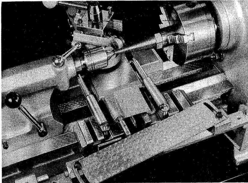
The "Viceroy" Copy and Taper Turning attachment has been designed as the result of requests from light industry and education authorities for a reasonable priced unit. It does not have the usual working parts found in conventional taper attachments and thus is easier to set and has less frictional losses.
