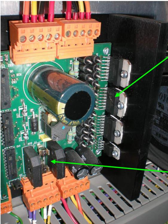
This is where the visible damage to the circuit board is. You just see that the plastic housing of the IC is damaged and this is also where the strongest smell of burning could be detected.
