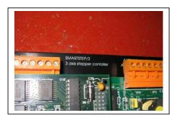
Identifying features: RED Seven Segment display SmartStep screen printing on base plate. Eight Orange Terminal blocks fitted to baseboard.
