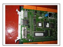
Identifying features: GREEN Seven Segment display CAM BUS Connector fitted between Display and RS232 connector Twelve orange connectors on base board
