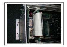
Identifying features: RED Seven Segment display Battery fitted between Display and RS232 connector
