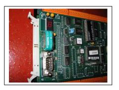
Identifying features: RED Seven Segment display Battery fitted between Display and RS232 connector Twelve orange connectors on base board
