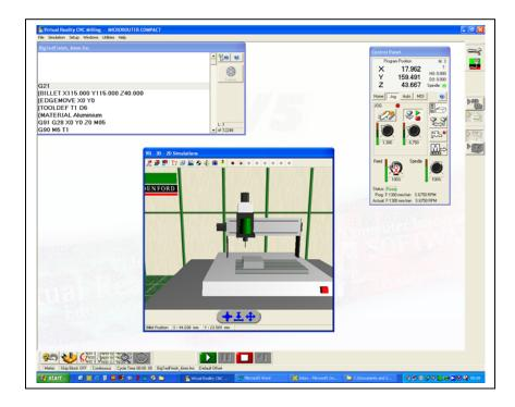
VR Milling 5 is the machine operating software supplied with the current Denford range of milling and routing machines.
