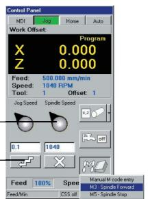
If you like you can go back to continuous jog and at approx 100mm/min jog the cutter in the X axis to 'Face-off' the end of the billet. Repeat this process until the end of the billet is flat (Perpendicular to the length of the billet).
