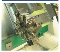
In the example pictured left, all the tool positions are occupied. A number of Boring Bars are fitted along with a Jacobs Chuck containing a drill.
