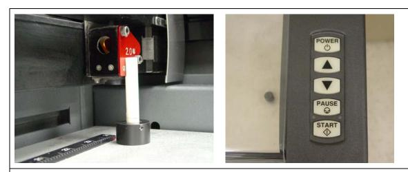
2. Using the UP and DOWN arrow buttons, either on the machine or in the VCP, bring the Z-axis table up. Using the appropriate Focus Tool for the lens installed (the standard is 2.0, other Focus Lens Kits are optional), focus directly on the surface of the table.
