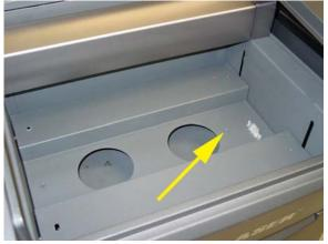
7. Lower the Z-axis table, halfway down. Loosen the two thumbscrews on the table and remove the table.
