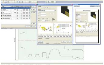
QuickTURN is an advanced yet simple to use, wizard based CAD/CAM package for Lathes. You can create or import 2D profiles, configure your tooling and material settings, then run the CAM wizard to create and simulate CNC Lathe toolpaths. The software features fully automatic toolpath generation, picking the most suitable tool from those available.
