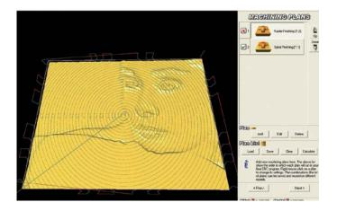
QuickCAM Pro is an advanced, yet simple to use, wizard based CAM package, which is used to create cutter paths for machining 3D parts on a milling machine or router. Both STL files and image files can be imported into QuickCAM Pro, and a comprehensive set of machining plans can be used individually or in combination to produce complex 3D surfaces and lithophanes.
