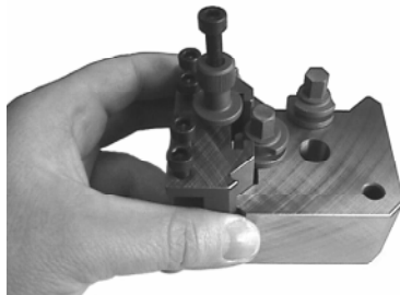
Slide the toolholder onto the toolpost...
