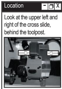
The two X axis slideways are located on the left and right sides of the saddle and cross slide. To lubricate the slideways, use the oiling points mounted on the upper right and left sides of the saddle, as shown below.
