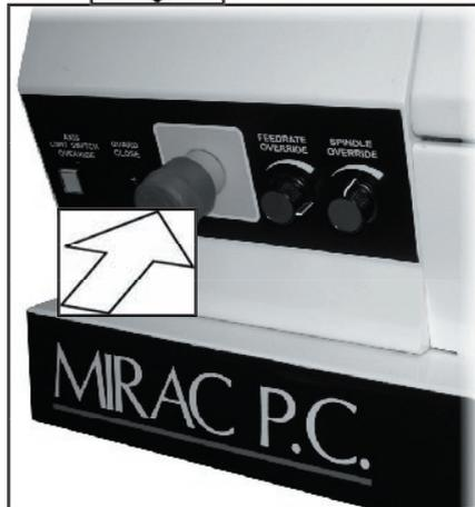
A circular, red emergency stop button is mounted on the front operators panel, positioned on the left side of the machine cabinet. When pressed, it has the effect of stopping all axis and spindle movements immediately. The interlock switch will also close. When the safety guard door is in its closed position, this will prevent access to the working area of the machine.
