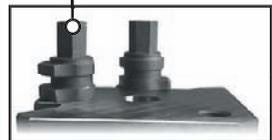
Double flanged locknut open (pointing towards the centre of the toolpost).
