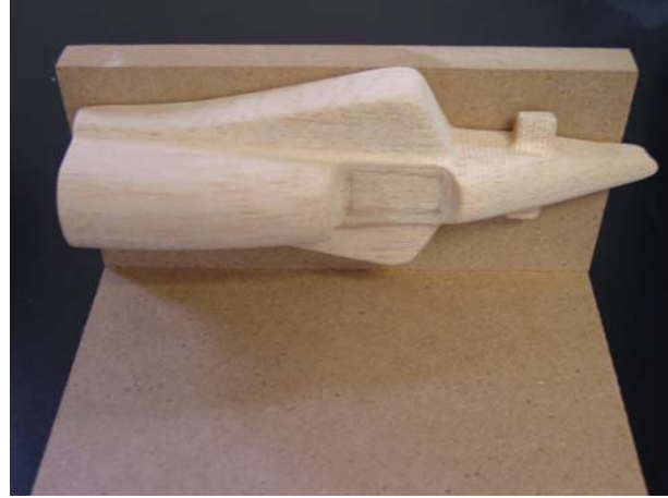
Figure 13 - Axle Drilling Fixture
