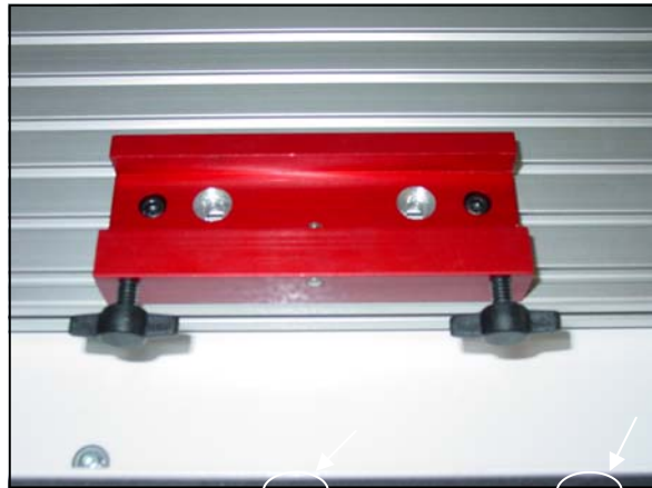
Figure 1 - The Fixture Base Plate.
