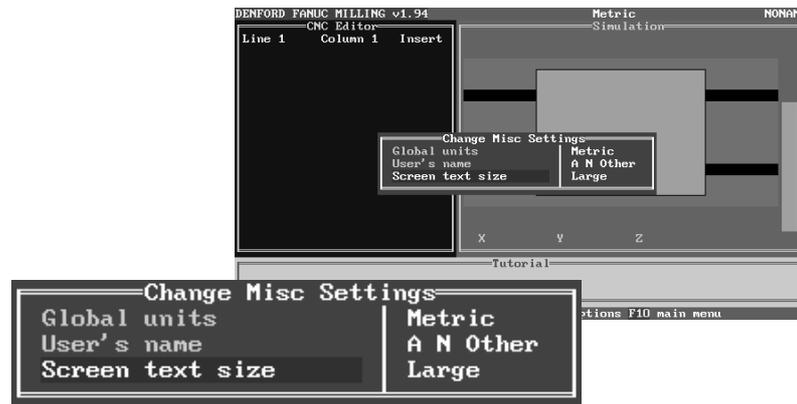
When set to '*Small*', the text size is set to 43 lines on screen :
