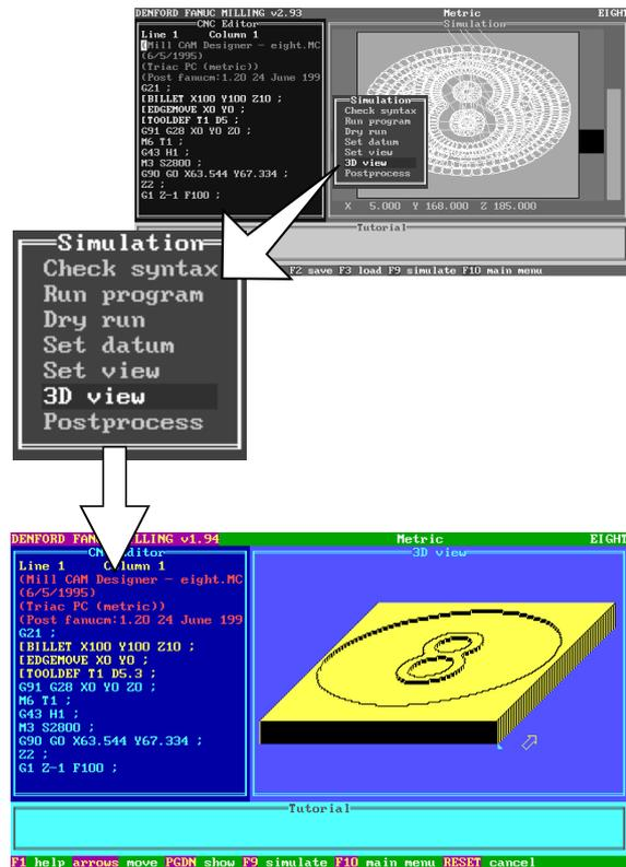
The [PAGE UP] key can be used to toggle between a back or front 3d view of the design.
