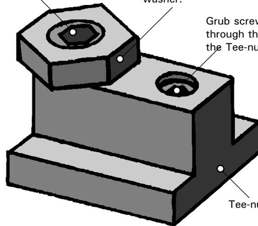
The base of the Miteebite clamp consists of a Tee-nut, with 2 threaded holes passing right through its section from top to bottom.
