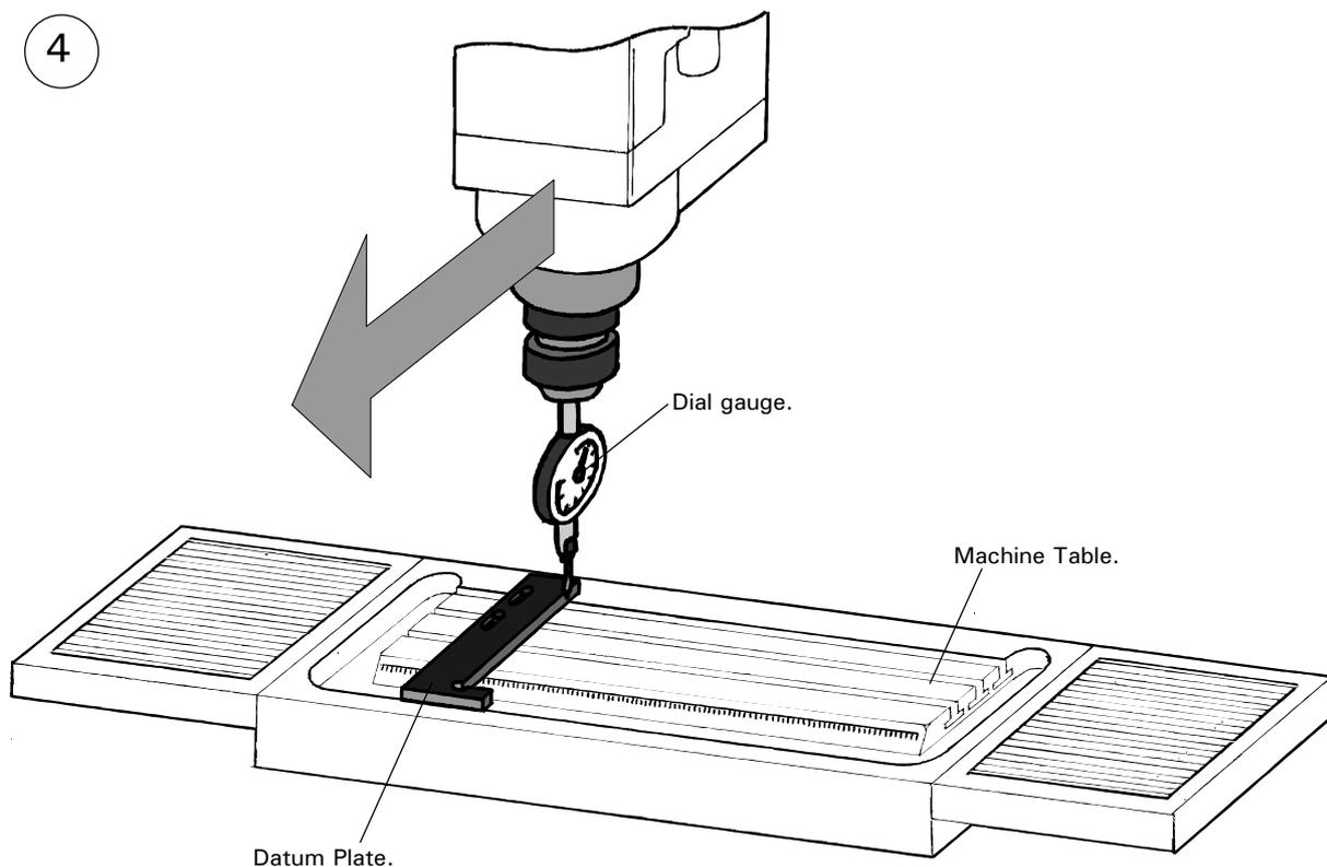
Set up the machine so a dial gauge is held in place of the cutting tool (the [T] key will change tools on an automatic tool changer). Align the dial gauge so it is positioned along one of the 2 sides of the datum plate, which run parallel with the Y axis. Use the [+X], [-X], [+Y], [-Y], [+Z] and [-Z] keys to move the dial gauge, with the *Jog Mode* set to read '*continuous*' on screen (this can be selected using the [JOG] key).
