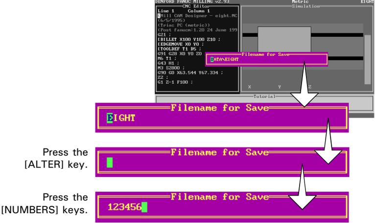
Press the [EOB] key to save this new file to the currently selected drive. Press the [RESET] key to clear the screen of any unwanted menus or information.
