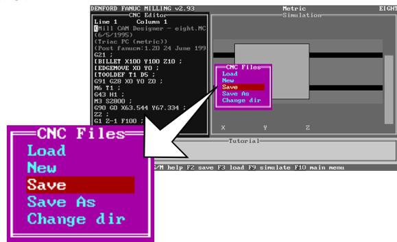
If the CNC File has never been saved, ie, it has just been manually entered, the software will prompt for a filename. Use the [NUMBERS] keys to write a filename into the dialog box. Incorrect characters can be removed using the [DELETE] key. Press the [EOB] key to save the CNC File.
