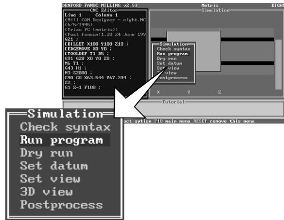
The '*Run Program*' option is set to run through the entire CNC File cycle, from start to finish. Whilst the CNC File is running, the written text will scroll down the screen and the pictorial view will be simultaneously updated.
