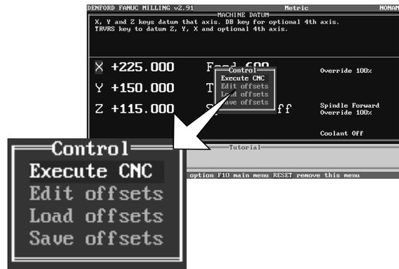
The machine will switch to *Auto Mode* and will allow the user to run the currently loaded CNC File.
