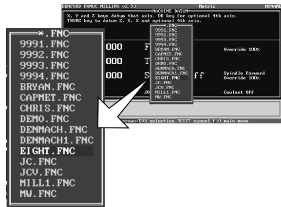
If there is a CNC File currently in the editor, the screen will display 'Do you want to merge?' (ie, do you want to combine the program you wish to load with the program already loaded). To merge CNC Files press the [Y] key, otherwise, press the [N] key to clear the current CNC File and load the selected CNC File into the editor.
