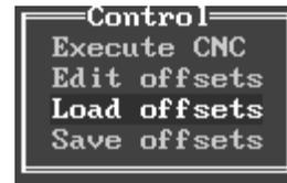
Note - the screen may display the previous setting for the drive. In the example below, the screen displays the drive as 'C:' , even though it has just been changed to load from 'A:' , as shown in the last section. If this occurs, press the [ALTER] key to reset to the new drive.
