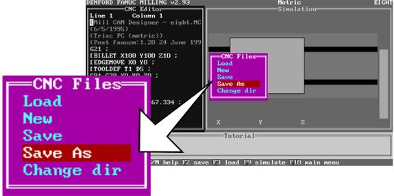
To remove the old filename, press the [ALTER] key, then enter the new filename using the [NUMBERS] keys. Any characters typed in by mistake can be corrected using the [DELETE] key.
