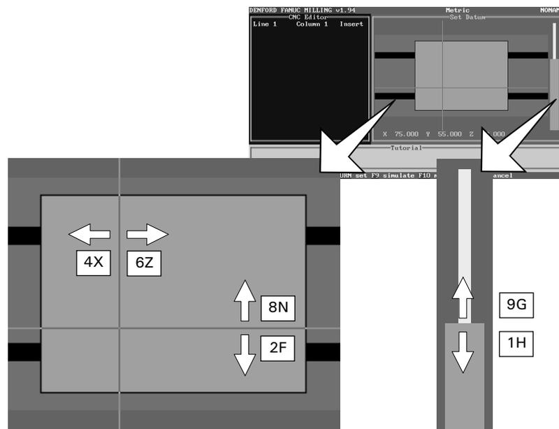
Press the [EOB] to set the graphical datum point, then the [RESET] key to clear any unwanted menus from the screen.
