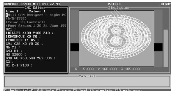
If the simulation window is set to display 3d views, the view editor will operate in plan view when the 'Set View' option is selected. The next time the CNC File is run, the 3d view will be that chosen in the view editor.
