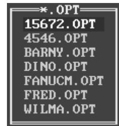
When the Setting File has been loaded, press the [RESET] key until all the menus have been removed from the screen.
