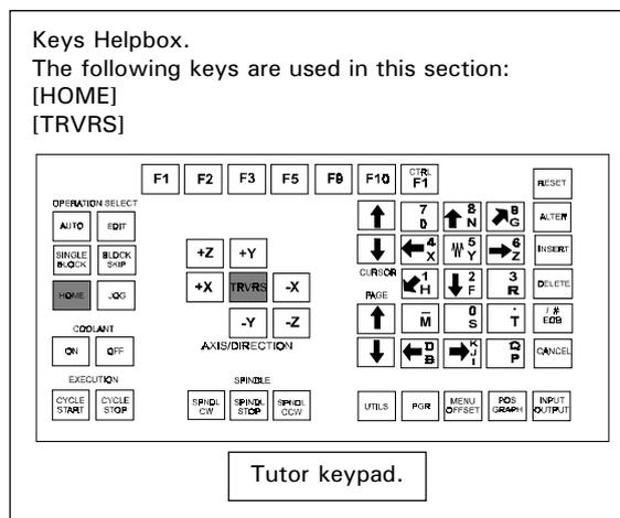
The helpbox above would show that the [HOME] and [TRVRS] keys are used at some point during that particular section.
