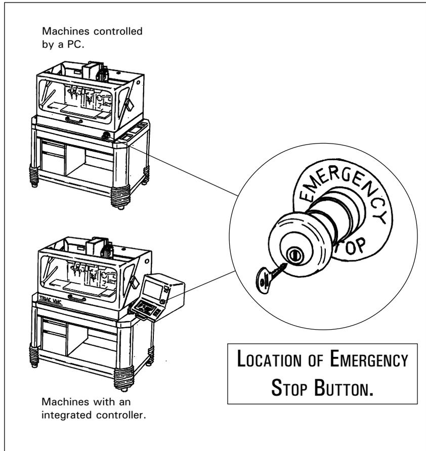
The red Emergency Stop button is located in two positions, according to the type of machine being used:
