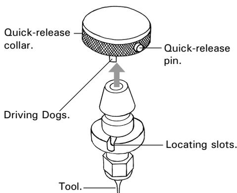
To refit, align the two locating slots of the tool with the two driving dogs on the quick-release collar. Push the tool up into the holder. The quick-release mechanism should now spring closed and grip the 'new' tool securely.
