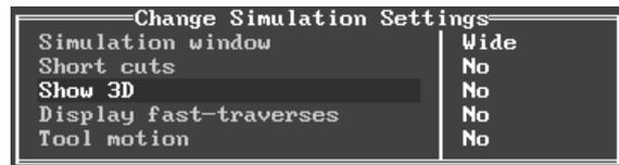
Now, when '*Run Program*' is selected, the work will be displayed in 3d, throughout the running of the program cycle.
