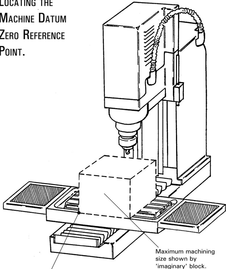
Front, left, lower corner of the block is the machine datum zero reference point, with the co-ordinates  $X=0, Y=0, Z=0$ .
