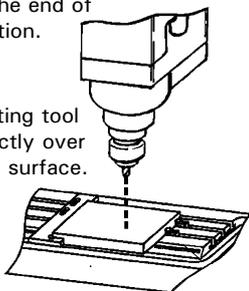
Select the *Jog Mode* by pressing the [JOG] key and check that it is set to '*continuous*'. Before moving the table in any direction, raise the head using the [+Z] key so that it is comfortably above any surfaces it could hit when moving across.
