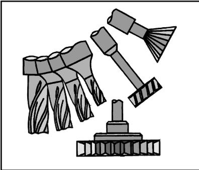
Each cutting tool is a different length, so the Z tool offset co-ordinates you have entered for tool 1 will not necessarily be correct when using other tool numbers.
