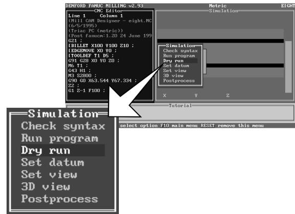
*Dry Run* will display any errors in your program, so if none are shown after pressing [EOB], your CNC program has run correctly. Error messages are displayed with the appropriate incorrect line in your program highlighted. Any error message windows which are displayed can be cleared by pressing the [RESET] key.
