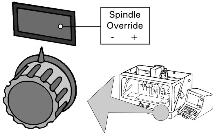
To increase the spindle speed, rotate the dial clockwise - as the dial is turned the 'faster' spindle speed will be updated and displayed on the control screen.
