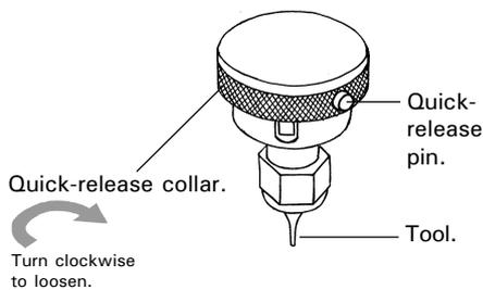
To physically remove a tool from the machine, grip the tool holder quick-release collar, so that the quick-release pin in it is fully depressed. Hold the tool itself still and rotate the quick-release collar clockwise until it stops. Remove the tool whilst keeping the quick-release pin still depressed - this prevents the quick-release mechanism from closing.
