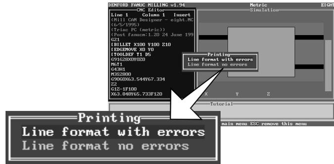
Press the [RESET] key to remove any unwanted menus from the screen.
