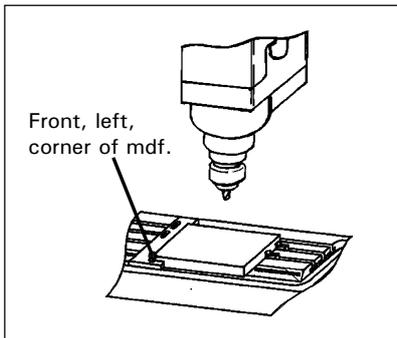
To set the X and Y co-ordinates, the position of the front, left, corner of the temporary MDF bed needs to be found.
