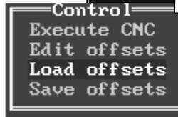
Enter the file name (number) for the offsets using the [NUMBER] keys and confirm this by pressing the [EOB] key.
