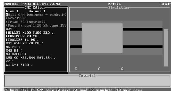
*Simulate only.* The CNC File can be simulated using a full screen graphical display(plan or 3d).
