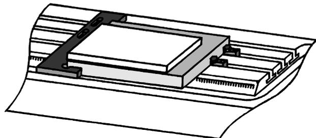
The actual workpiece, such as a sheet of plastic, would be held in place on the temporary MDF bed using double sided tape.
