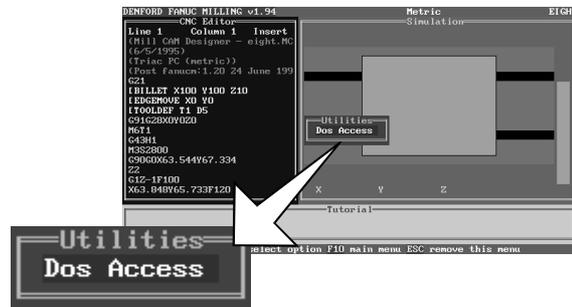
Other external DOS programs can be run when the computer is set in DOS mode. To return to the control software, type '*EXIT*' at the DOS prompt, then press the [EOB] key, when prompted.
