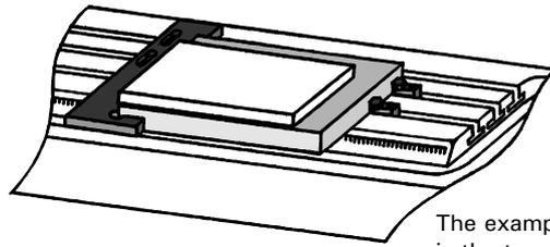
The example used in this section is the temporary MDF bed with a sheet of plastic retained using double sided tape.
