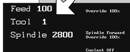
The spindle speed can be decreased down to a minimum value of 50%. To decrease the spindle speed, press the [DOWN KEYPAD ARROW] key until the desired value is displayed on screen.
