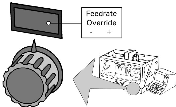
To increase the feedrate, rotate the dial clockwise - as the dial is turned the 'faster' feedrate will be updated and displayed on the control screen.
