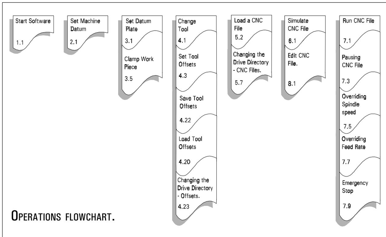
The Operations flowchart lists the progress of a typical operating procedure for a Milling Machine or Vertical Machining Centre. Sections in this manual correspond to each of the operations listed above.
