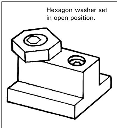
Now tighten the grubscrews in each miteebite to lock them firmly in position. At this stage, it should still be possible to remove the temporary MDF bed.
