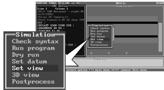
Press the [JOG] key to cycle through the different views. To select the view highlighted press the [EOB] key.
