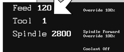
The feedrate can be decreased down to a minimum value of 0%. To decrease the feedrate, press the [LEFT KEYPAD ARROW] key until the desired value is displayed on screen.
