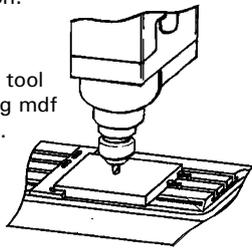
Using the [+Z] and [-Z] keys, make the tip of the cutter just touch the top surface of the bed.
