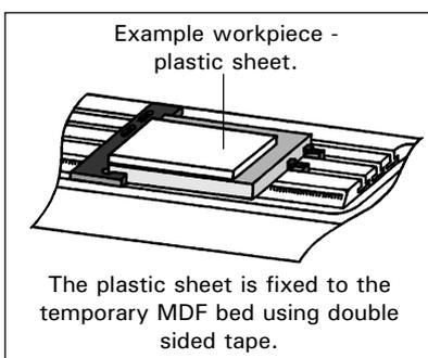
Now that the Tool Offsets have been set to coincide with the surface of the temporary MDF bed, the workpiece is fixed into position (in this example it is a sheet of plastic - refer to the diagram opposite). If the miller starts cutting it will take all its Z co-ordinate measurements from the surface of the temporary MDF bed (i.e. the Z Tool Offsets).
