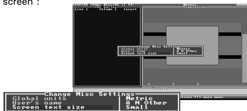
To select this option, highlight '*Screen Text Size*' using the [CURSOR ARROWS] keys and press the EOB] key. Continual pressing of the [EOB] key will toggle the option between the two settings.
