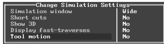
Now, when '*Run Program*' is selected, the tool motion will be shown, throughout the running of the program cycle. The program cycle will run considerably slower with this option switched 'on'.
