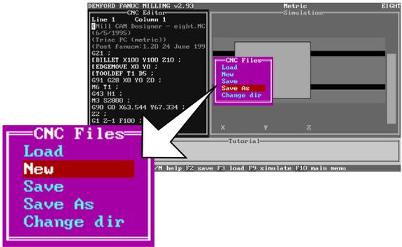
The current CNC File is cleared leaving the editor with no CNC File loaded.
