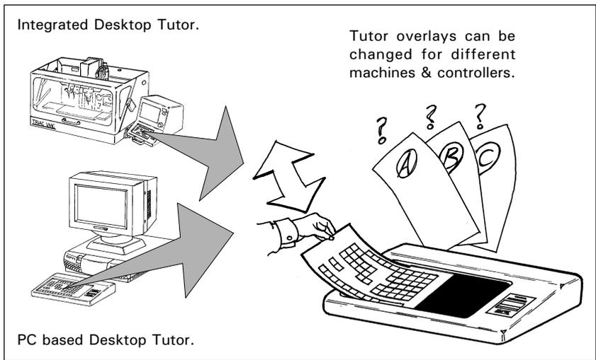
The Denford Desktop Tutor is the keypad input controller for the machine (i.e. the equivalent to a Qwerty keyboard on a pc), common to both pc driven and integrated machines. The overlays on Desktop Tutors are interchangeable, according to the type of machine and control method required.
