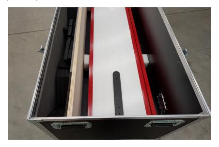
It is important to remove the track sections carefully and place the track spacers back in the case for re-packing the tack after use. The track legs and leg braces are stored in a separate padded compartment within the packing case and can be easily removed.
