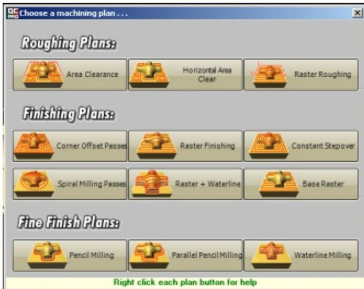
Here you have a choice of 3 roughing plans, 6 finishing plans, and 3 fine finishing plans. Right clicking each plan will launch a help file to describe how each plan works. For this tutorial we will use a Raster Roughing, a Raster Finishing, and a Pencil Milling plan.
