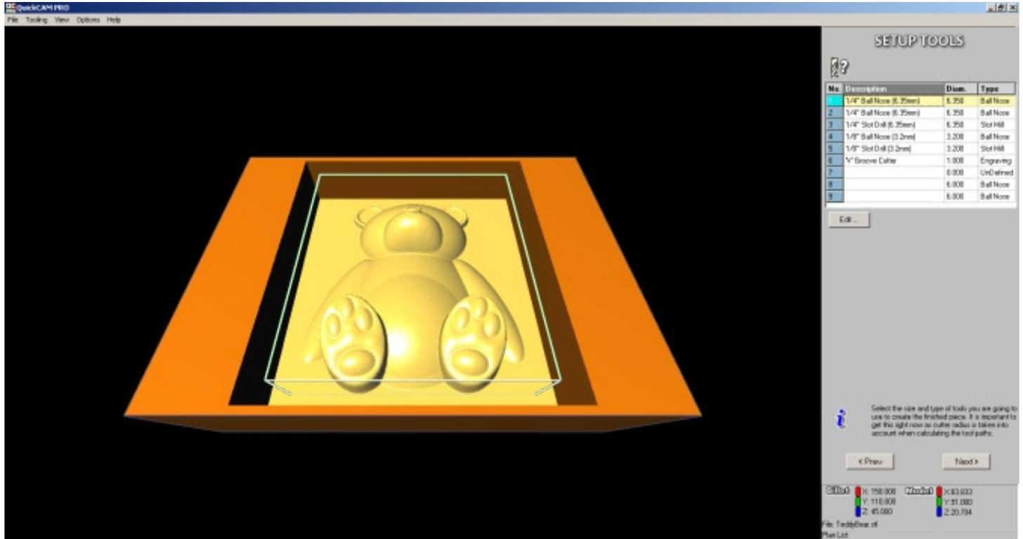
This screen takes the tooling information from VR Milling V5, as long as you have set the 1/4" Ball-nose in VR Milling V5 it should be showing here.
