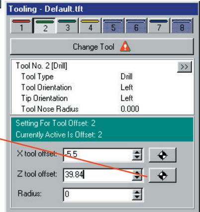
When the 'Z Offset' window appears there will be a value in the 'Distance to origin' dialogue. This is the distance the machine has to travel to reach the billet, relative to Tool 1. If the machine has to travel further it will be a negative number, if it has to travel less it will be a positive number.
