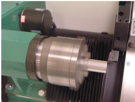
If you like you can go back to continuous jog and at approx 100mm/min jog the cutter in the X axis to 'Face-off' the end of the billet. Repeat this process until the end of the billet is flat (Perpendicular to the length of the billet).
