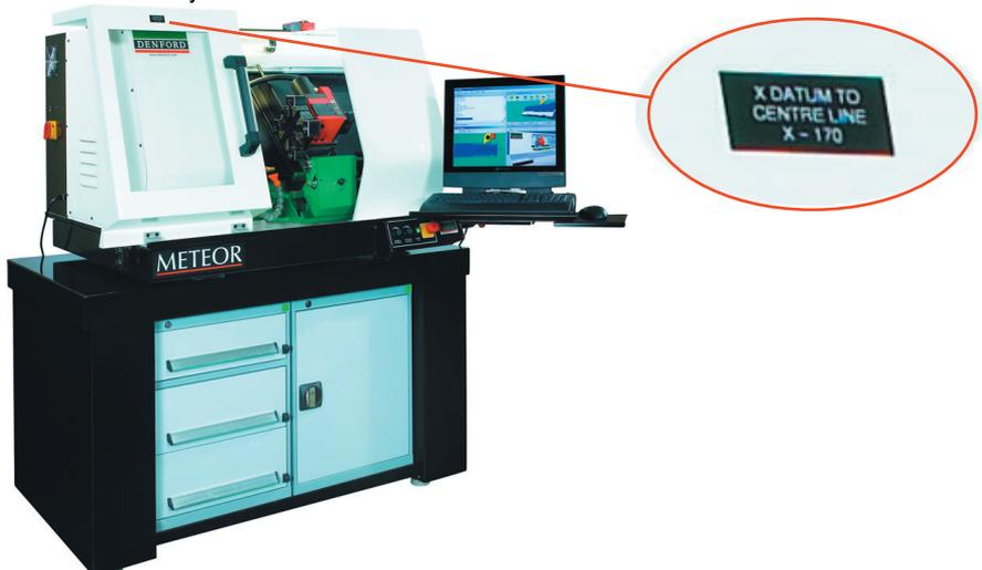
If using a Meteor, Mirac or Cyclone click the datum button next to the X tool offset dialogue box within the 'Tooling' window.
