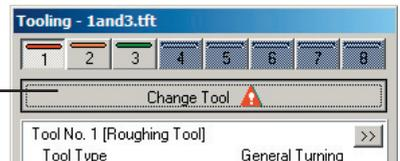
If your machine has an ATC the tool post will traverse to the tool change position, then rotate to change the tool.
