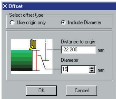
The 'X Offset' window will open. In the top dialogue box is the distance the tool has travelled from it's Home position to its current position.
