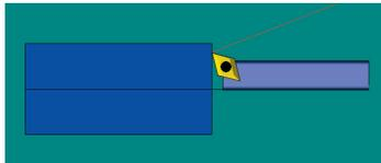
Click the Datum Button in the 'Tooling' Window and set the 'Z tool offset'.
