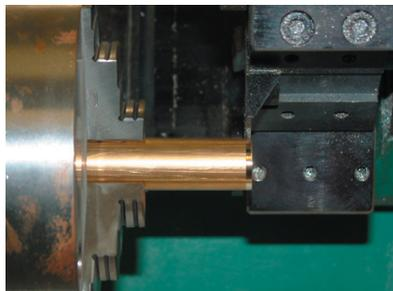
Change tools to the Threading Tool as described in 'Step 8' of this guide. In this example we have the Threading Tool set as Tool 7.
