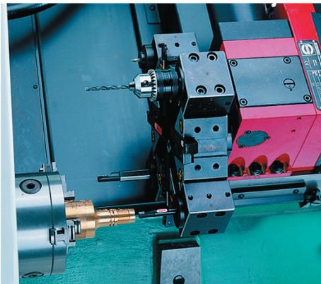
In the example pictured left, all the tool positions are occupied. A number of Boring Bars are fitted along with a Jacobs Chuck containing a drill.
