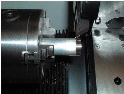
Go back to continuous jog and at approx 100mm/min jog the cutter in the Z axis to 'Turn down' a section of the diameter of the billet.
