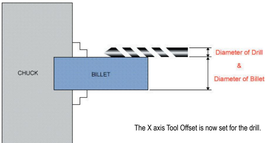
The X axis Tool Offset is now set for the drill.
