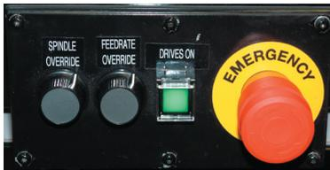
If necessary release the Emergency Stop button. On some models it you will need to press the 'Drives On' button to enable the drives. (On most machines the drives power up automatically)
