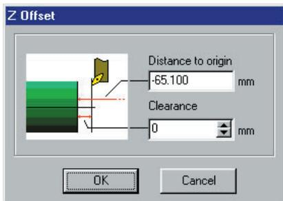
The 'Z Offset' window will open. In the top dialogue box is the distance the tool has travelled from it's Home position to its current position.
