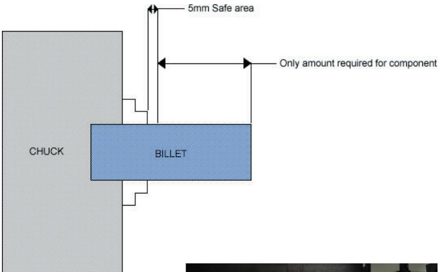
You will have to measure the amount of material protruding from the jaws of the chuck.
